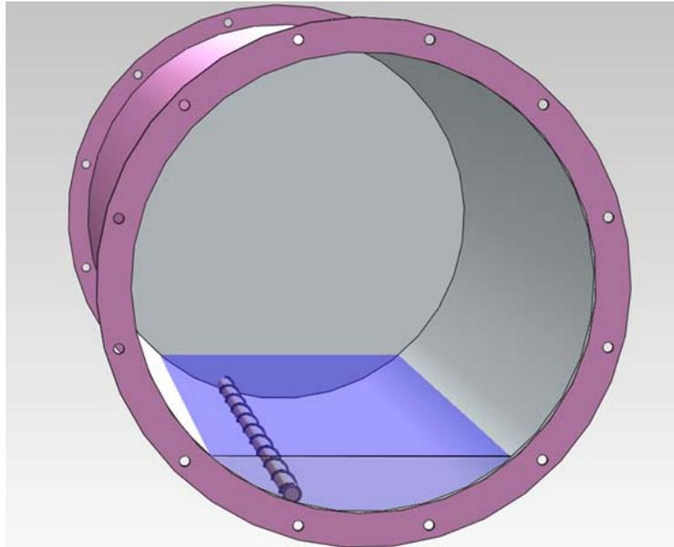
Figure 2 - Example of the system of continuous cleaning of the heating surfaces from salt deposits using rolled rod with cleaning edges
