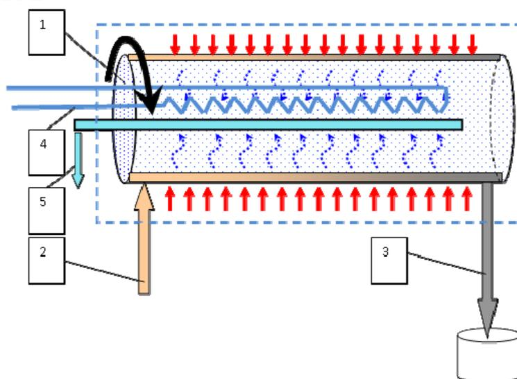
*Figure 1. Diagram of the evaporation treatment of the liquid radioactive waste in the DFE: 1 - drum evaporator; 2 - supply of initial solution; 3 - discharge of the concentrate; 4 - secondary steam condensation circuit; 5 – secondary steam condensate discharge*
