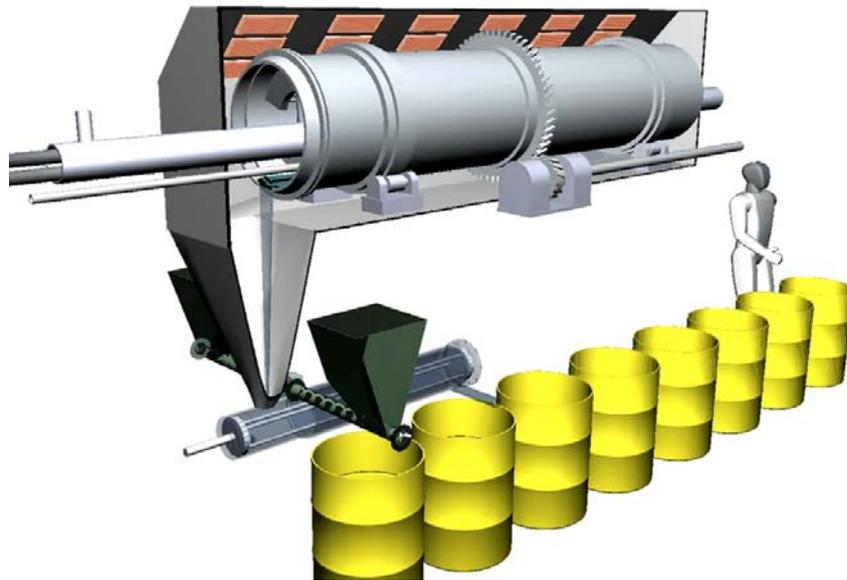
*Figure 6. Continuous technological process of vat residue secondary evaporation in electrical heated DFE and concentrate conversion into cement compound*
