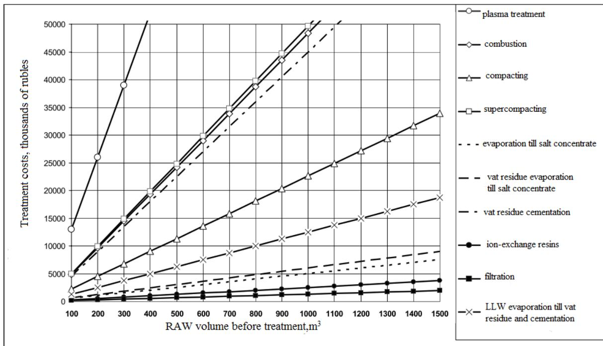
Figure 5. The cost of RAW preparing for final disposal, depending on applied technical solutions
