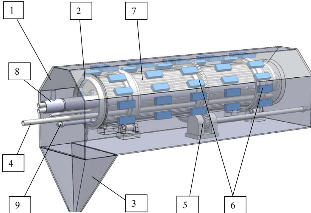
*Figure 2. Scheme of the main components of drum-film evaporator:
